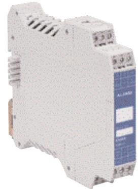
The IQ8TAM technical alarm module is connected as a BUS user to the analog loop of fire alarm systems 8000 and IQ8Control and allows acquisition, transmission and single indication of technical alarms. Since voltage is supplied via the esserbus, individual voltage supply is not required.
